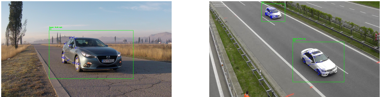
FIGURE 5: Sample image from the VS13 dataset (left) and BrnoCompSpeed dataset (right), annotated using the speed estimation framework.
