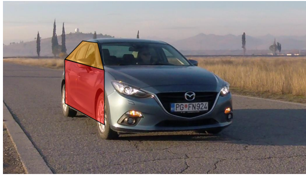
FIGURE 1: Piecewise planar approximation of a vehicle body. (Frame sampled and modified from the VS13 dataset (Djukanović et al. 2022)).
