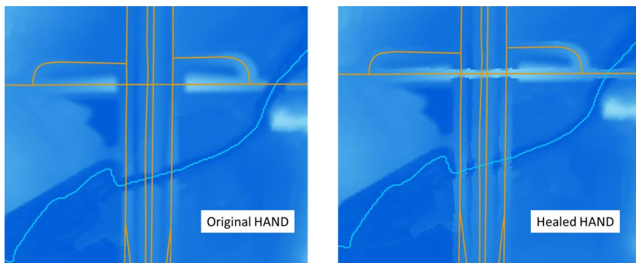
Figure 8 Healing the Height Above Nearest Drainage for Missing Bridge Structures
