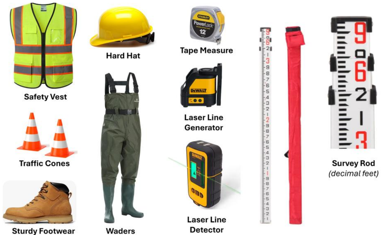
Figure 8. Example equipment for survey field work.
