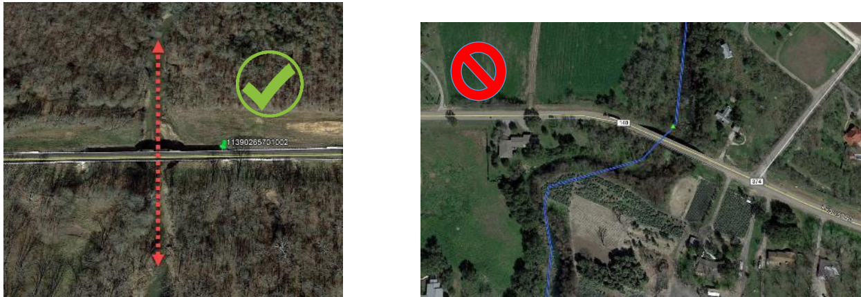
Figure 4.1. Examples of straight vs. curved stream reaches at bridges.
