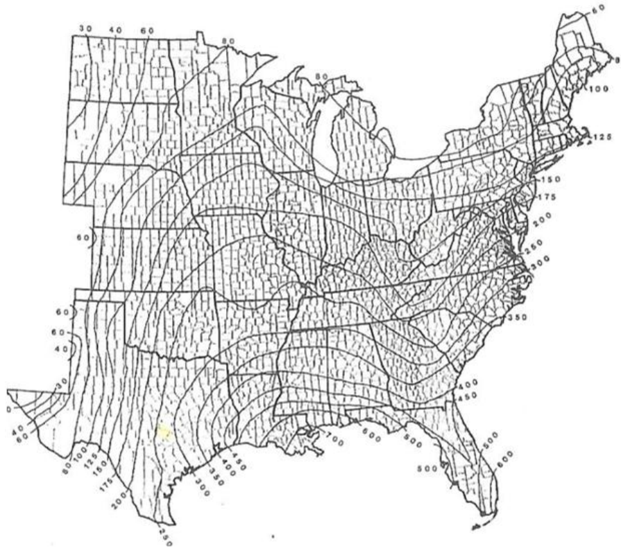
Figure 2. Adapted from Haan et al. (1994), Isolines of annual R factor for the Eastern United States (ft•tonsf•in/acre•hr•year)
