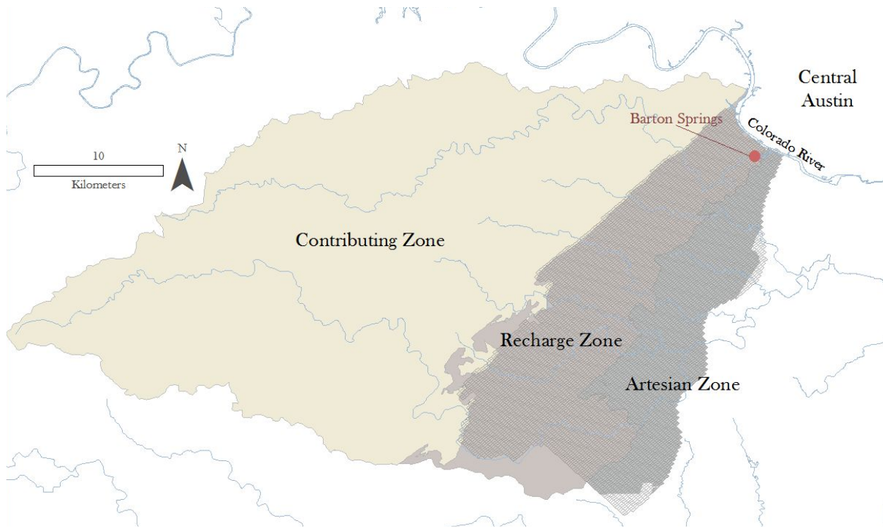
Figure 2 Extent of MODFLOW model active cells in the Barton Springs segment of the Edwards Aquifer. The model contains 7036 active cells at 500 feet by 1000 feet per cell.
