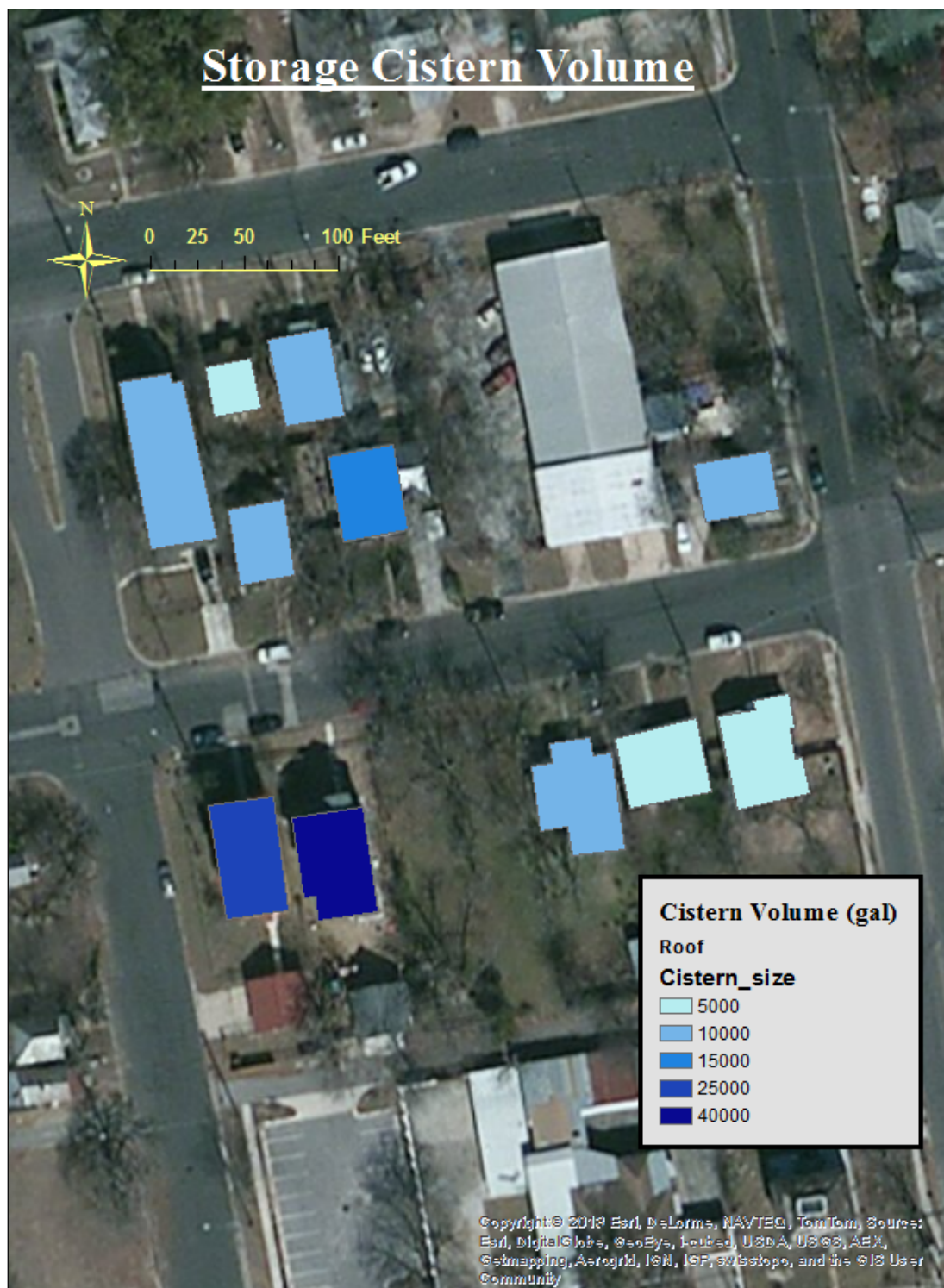
Figure 4: Storage Cistern Design for Case 2
