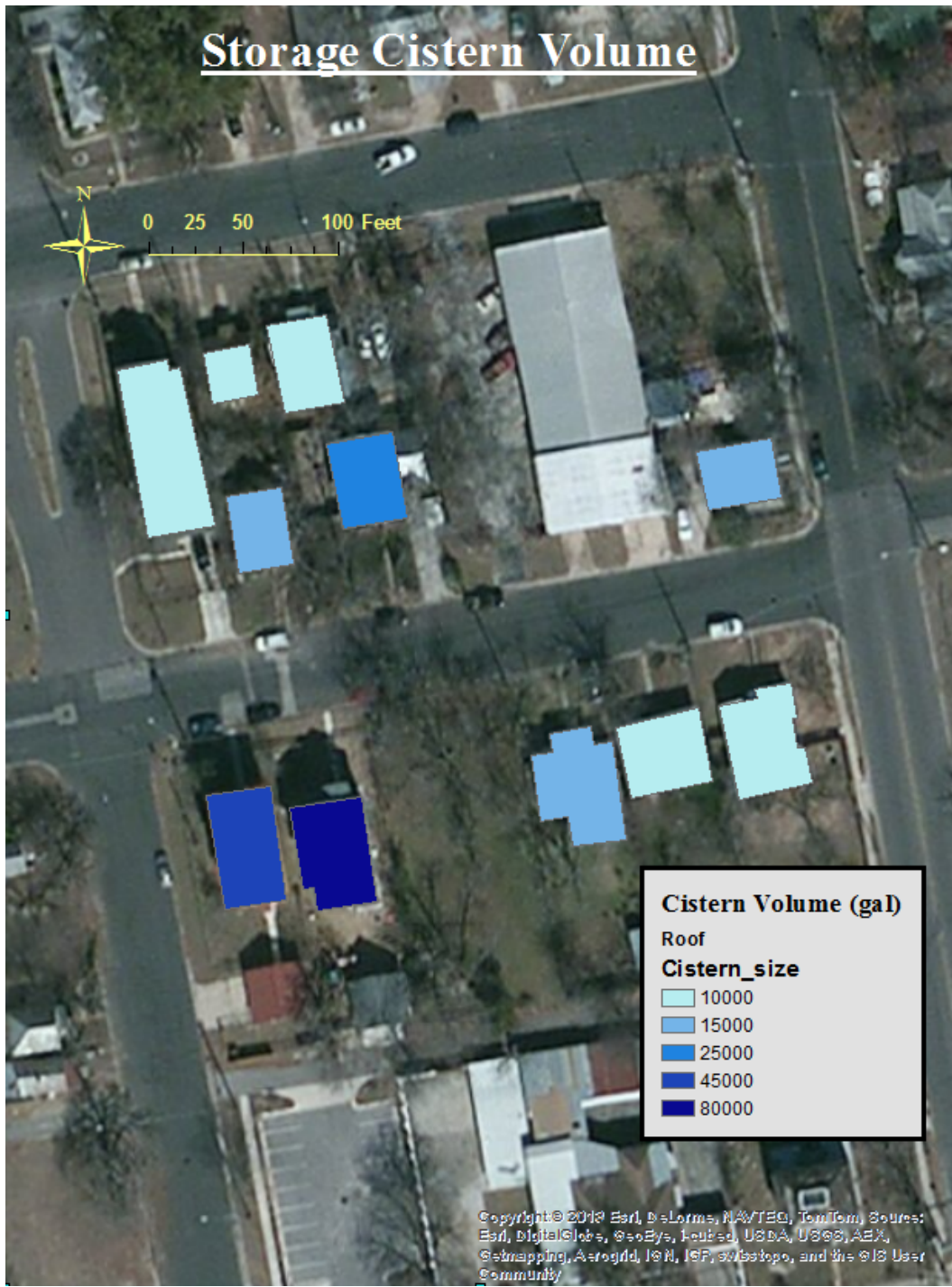
Figure 3: Storage Cistern Design for Case 1
